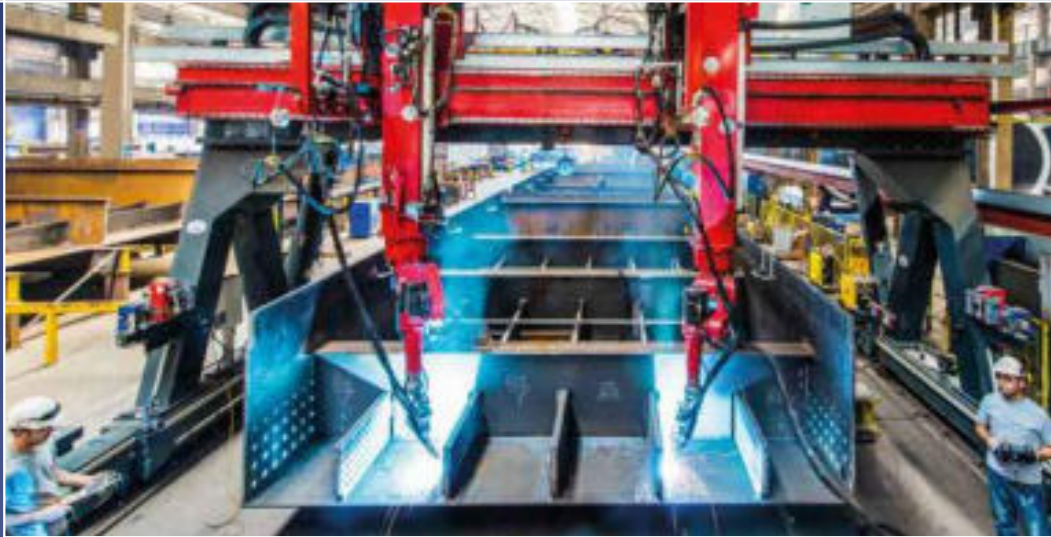
TOWER PANEL FABRICATION
