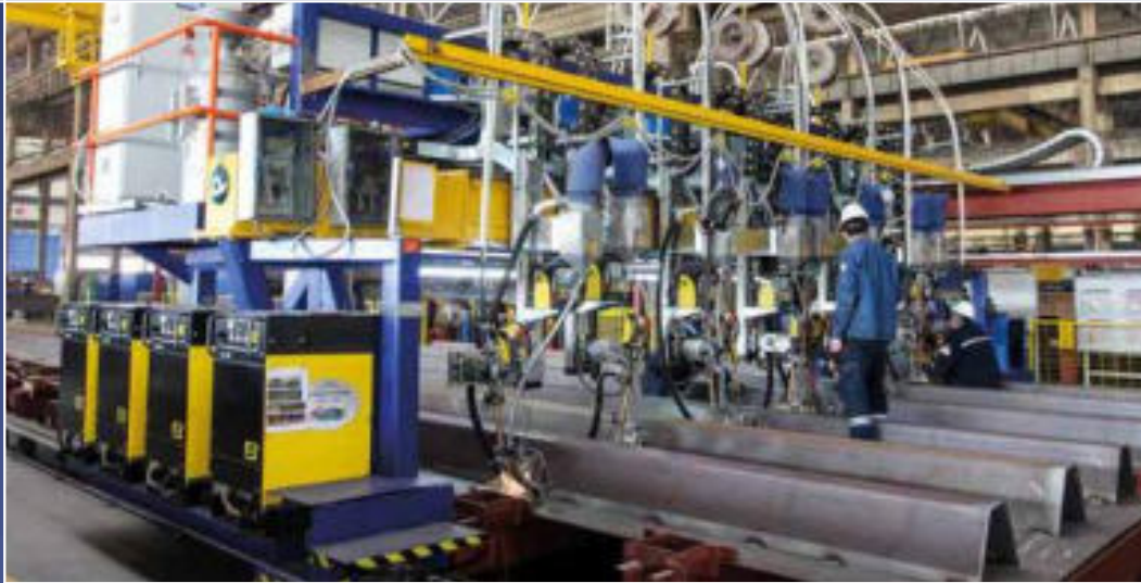
GIRDER PANEL FABRICATION
