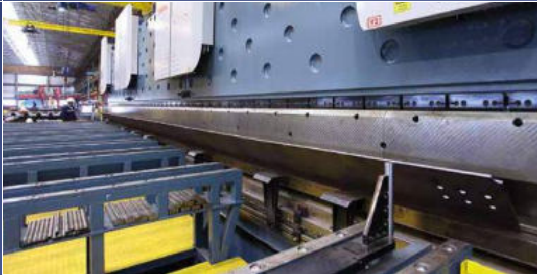
CNC PLATE - PROFILE BENDING
