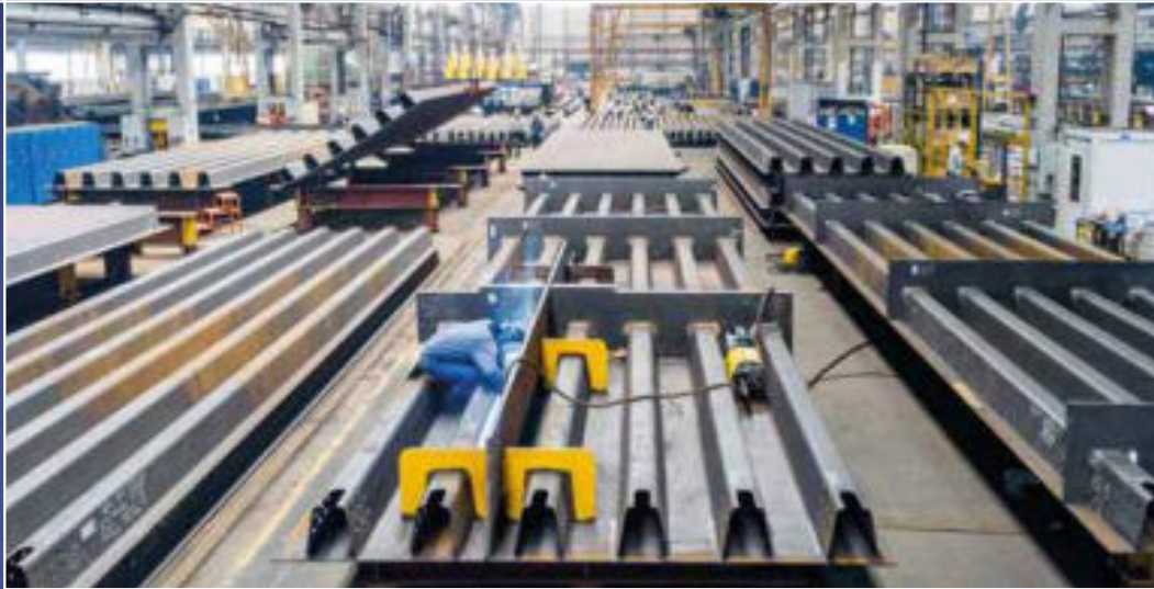
GIRDER PANEL FABRICATION
