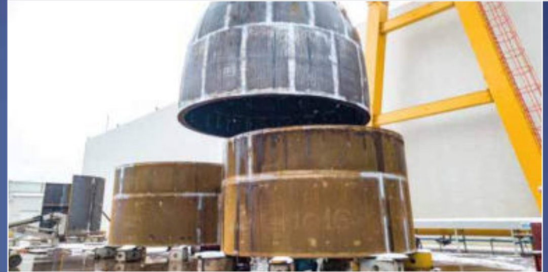
TOWER TOP ENCLOSURE TRIAL ASSEMBLY
