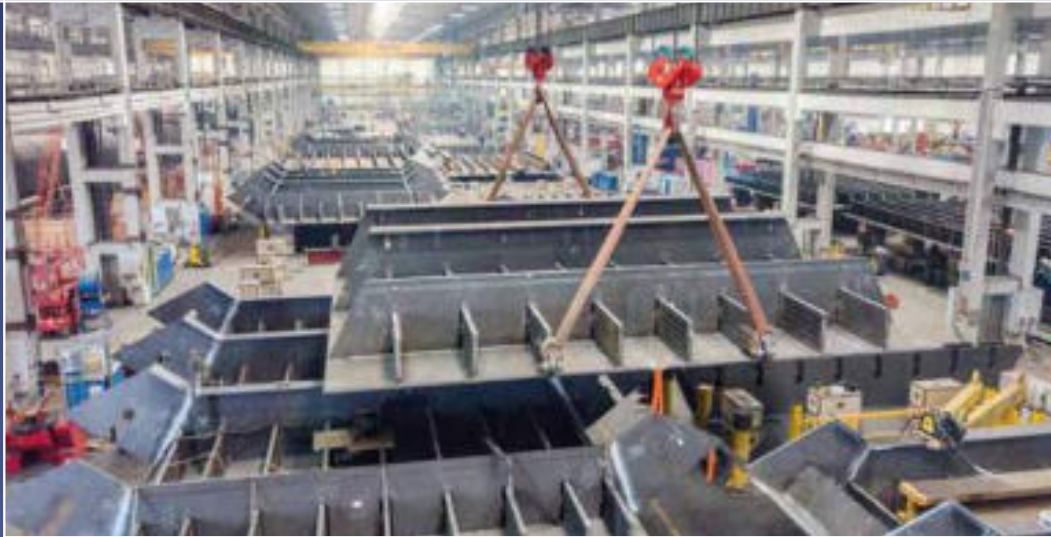
TOWER PANEL FABRICATION
